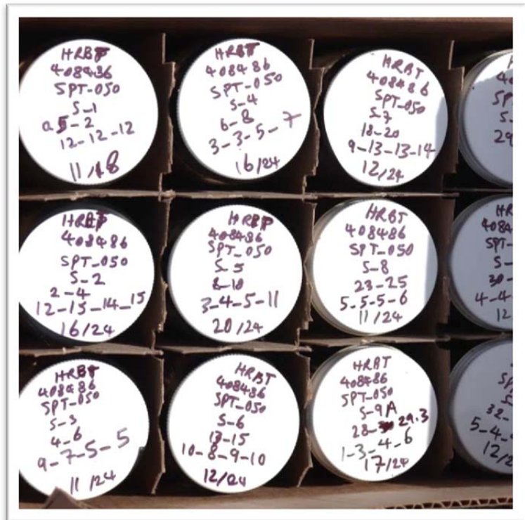
Soil samples from South Island, stored in protective cases prior to testing, to provide data for bored tunnel design
